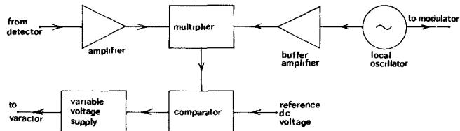
Fig. 2. Block diagram of the electronic control circuit.
