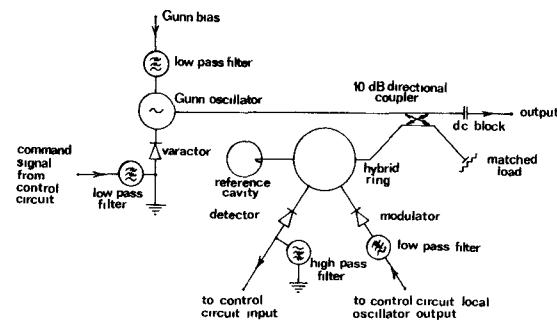
Fig. 1. Schematic diagram of a modified Pound stabilized MIC Gunn oscillator.
